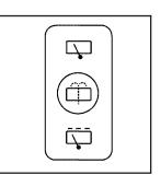
If your vehicle has a rear window wiper, the switch is located on the center console. See *Instrument Panel Overview on page 168*.
